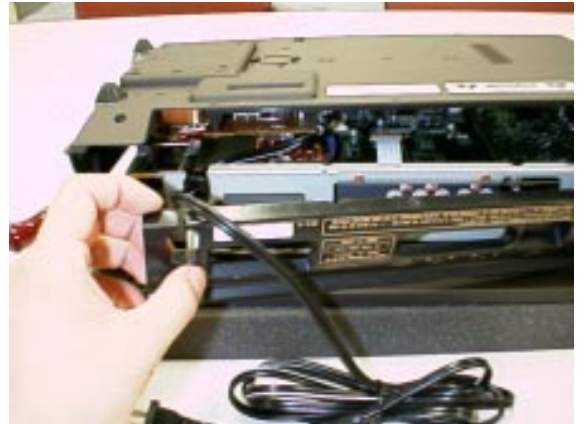
Fig.6 Removing the rear panel
