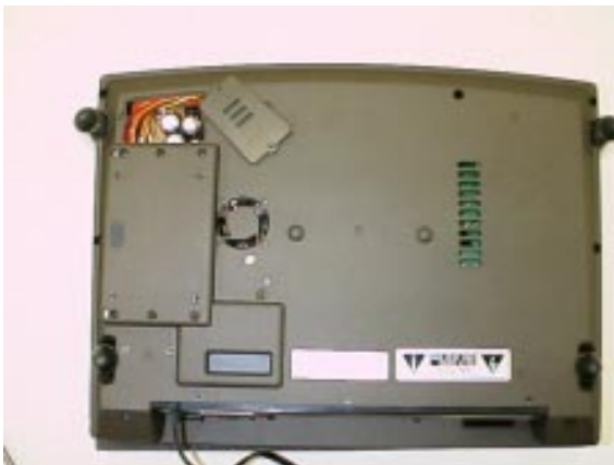
Fig.9 Removing the lid of the bottom case
