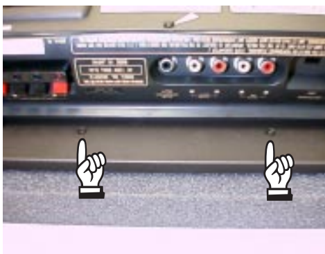
Fig.13 Pushed the rear panel
