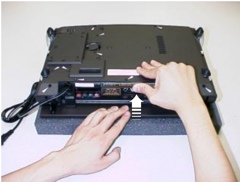
Fig.11 Pushing the rear panel
