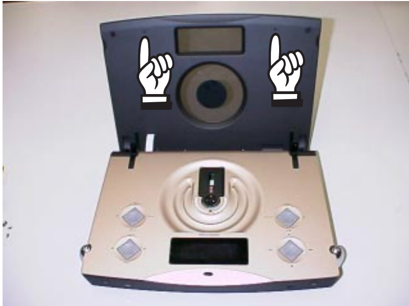
Fig.15 Positions of 2 screws on the top
